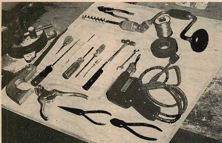
Fig. 1. What the amateur audio constructor should have handy in tools and accessories. Note the reel of resin core solder and insulating tape. Item to left of long-nosed pliers is a wire-stripper. Stickleback saw is between the keyhole saw and wire stripper.
