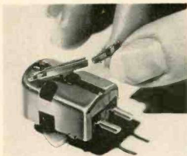
Latest model of G. E. Triple Play cartridge has simplified method for changing styli.
