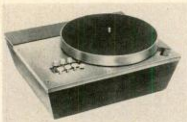
Scott Stroboscopic Turntable uses push buttons to select speed, has vernier adjustment for each of the three speeds.
