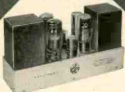
AA-904 PILOTONE AMPLIFIER World famous Ultra-linear Williamson circuit — an electronic triumph characteristic of the wide range of Pilotone Amplifiers.
