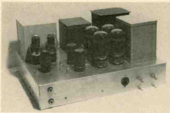
Fig. 2. Amplifier and power supply are together on the 13 × 17 × 3-inch aluminum chassis. Steel might be a better chassis material if the unit is to be handled to any extent.
