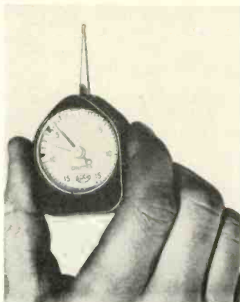
Scheer stylus-force gauge gives accurate dial indication between 2 and 15 grams.
