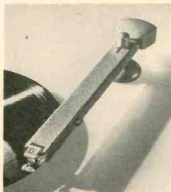
Pickering arm; cartridge mounting plate is hinged near front and offset for proper tracking.
