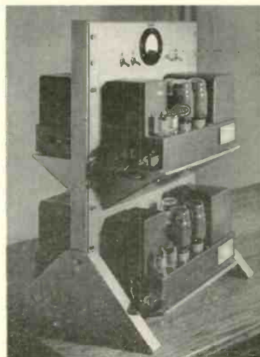
Fig. 3. The four standard QUAD amplifiers were mounted on this small rack.
