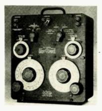
useful for measuring the impedance-frequency characteristics of such devices as electro-acoustic transducers, capacitors, transformers, and filters. Manufactured by General Radio Company, 275 Massachusetts Ave., Cambridge 39, Mass. P-12
