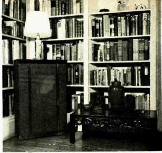
Fig. 3. Heard with "presence" but not seen is the 12-inch duplex Stentorian speaker with 11½ pound magnet. Plenty of excursion for clean lows through Cabinart's KR-4 Klipsh-designed folded horn, and tweetered to highs with separate coaxial-mounted voice coil. (The camera "saw" the speaker, but we are not a camera!)
