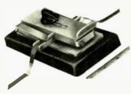
splice is trimmed parallel to the tape with a "Gibson girl" shape—two concave cuts made in the tape edges. Tape ends to be spliced are held in the tape guide by pressure fingers. The unit is mounted on a heavy cast base for bench use, but may be removed from the base and mounted directly on a recorder. Manufactured by Robins Industries Corporation, 41-08 Bell Blvd., Bayside 61, N. Y.
