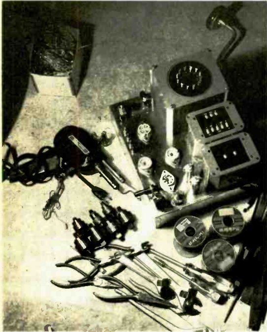
Fig. 3 (above). Dual amplifier system interconnected with filter network (small chassis in foreground). Left, array of 60-watt low-frequency power amplifier with power supply; right, 40-watt high-frequency array. Note two Mullard EL34's on this power amplifier.
