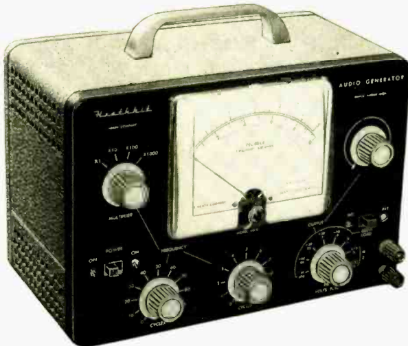
Fig. 5. Heathkit AG-9 Audio Generator, with step-type switching for selection of output frequency.
