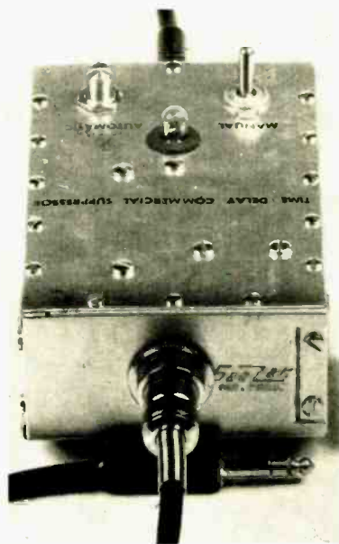
Fig. 5. Rear view of suppressor chassis shows use of Amphenol plug for connection from amplifier.
