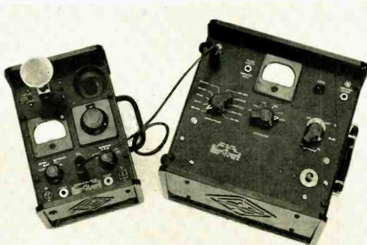
Fig. 9. Illustrating ease of interconnecting octave band wave analyzer to noise level meter. (General Radio Co.)
