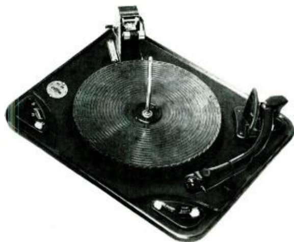
Fig. 1 (left). The Garrard RC-88 "Triumph II" automatic record changer—similar to its predecessor, the RC-80, but improved throughout. Fig. 2 (below). The RC-98, offers several deluxe features—most outstanding being the vernier speed control, actuated by the knob at the left of the turntable.
