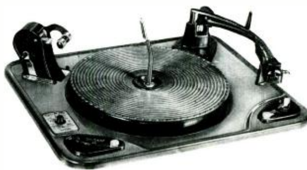
Fig. 1 (left). The Garrard RC-88 "Triumph II" automatic record changer—similar to its predecessor, the RC-80, but improved throughout. Fig. 2 (below). The RC-98, offers several deluxe features—most outstanding being the vernier speed control, actuated by the knob at the left of the turntable.
