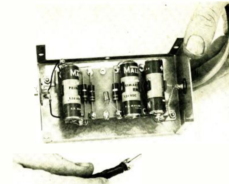
Fig. 3. Close-up of internal construction. Battery clips specified in parts list eliminate need for soldering batteries in place.
