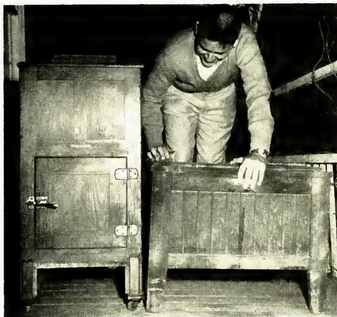
Fig. 5. The author starts to work on a second set of cabinets. Heavy and solid construction make the ice box equally suitable for loudspeaker housing.
