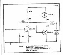
Fig. 13. Complementary-symmetry output stage.
