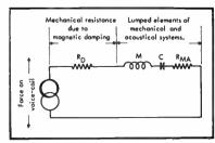
Fig. 2. Simplified electrical analogy to mechanical system of a speaker, including the mechanical resistance introduced by magnetic damping
