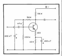
Fig. 11. Temperature-compensated transistor stage.
