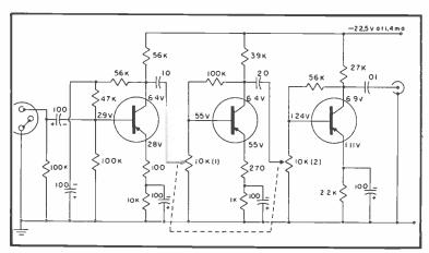
Fig. 12. Experimental microphone amplifier,
