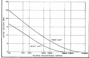
Fig. 3. Noise factor vs. source resistance for type vacuum tubes.
