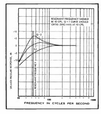
Fig. 1. Response of a direct-rodiator speaker system, in the region of resonance, at different values of Q of its mechanical system, (After Beranek)
