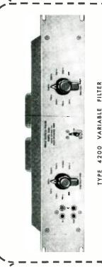
Eliminates the need for special precautions against hum pickup in circuits having signal levels as low as -40 dbm. Negligible intermodulation distortion at levels up to +20 dbm. All capacitors and inductors hermetically sealed for lifetime service. Aging effects are negligible. Requires only 3½" rack space.
