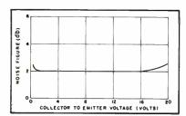
4. Variation of noise figure with collector-to-emitter voltage.
