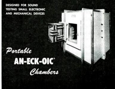
Model #545-250 as shown (outside dimensions 65" x 541/2" x 65", interior free field dimensions 33" x 22" x 33") is designed for a low-frequency cut-off of 250 cps. Chamber is mounted on Korfund spring vibro-isolators.
