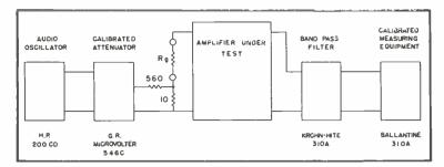
Fig. 14. Noise-figure measurement setup.
