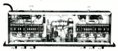
Fig. 7. Bottom view of completed amplifier chassis.
