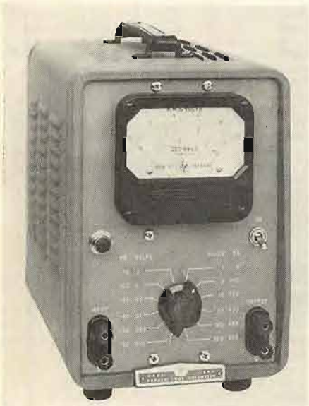
Fig. 6. A typical audio voltmeter. Although the scale is marked "Decibels," the reference level indicated on the meter is given as 1 mw/600 \Omega . Observe that 0 on the db scale is directly under 0.775 volts on the rms voltage scale. The meter is in reality a dbm meter. (Courtesy Hewlett-Parkard Co.)
