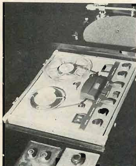
Fig. 1. View of the "well" containing portable Ampex A-122 tape recorder.
