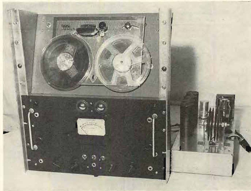
Fig. 6. The tape deck is attached to the amplifier by means of two "Tee" bars. Although the power supply is shown next to the amplifier it should be no closer than three feet when it is being used.
