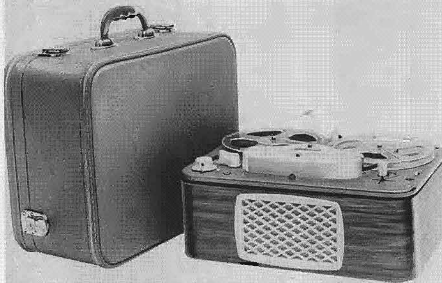
Fig. 2. Tandberg's new model 5-2 is similar in appearance to the earlier models, but offers four-track stereo performance.
