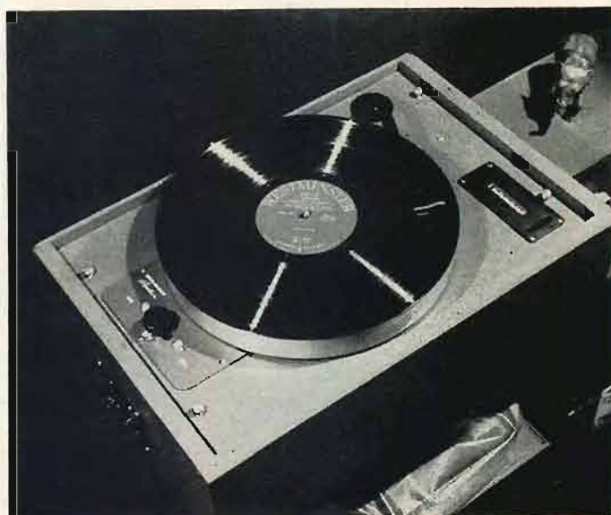
Fig. 2. Top view of turntable showing flush mounting of counter.
