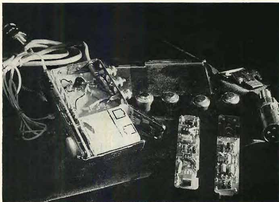
Fig. 5. Completed amplifier with some of the component parts shown separately.
