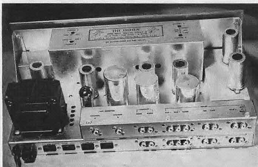
Fig. 4. Chassis view of the Fisher 400-C shows input jacks, level-set controls, and general layout.
