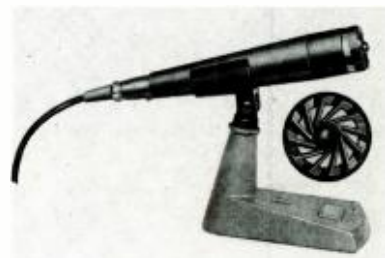
Fig. 13. The cardioid microphone with its housing and holder.
