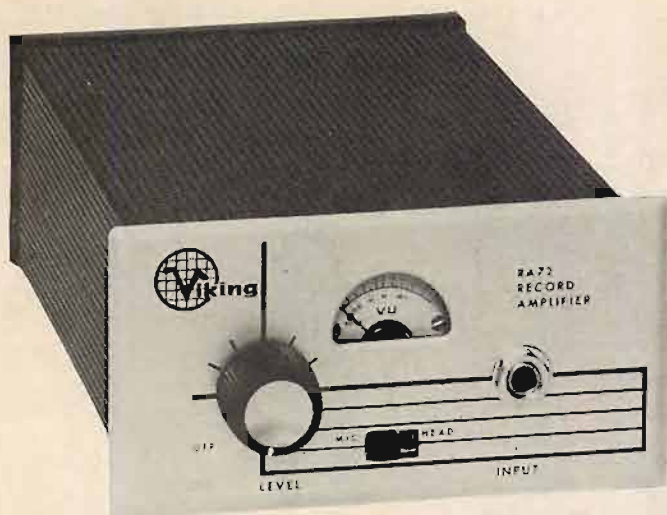
Fig. 5. One of the two RA72 recording amplifiers used in the Stereo Compact.
