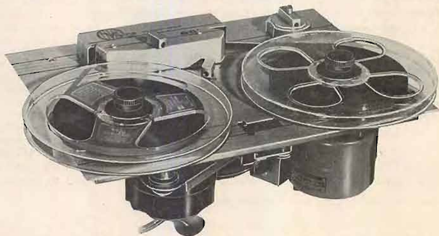
Fig. 4. The Viking 85-Series transport which is a part of the Stereo Compact.
