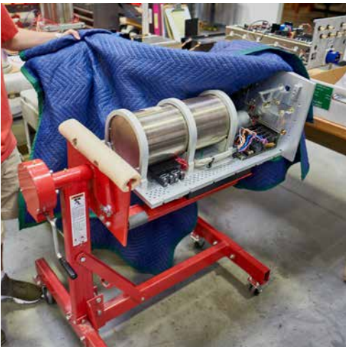
Boulder uses a fully rotating automobile engine stand to work on their amplifiers. WOW!
