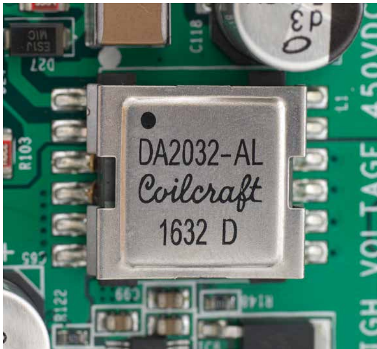
A high-quality Coilcraft transformer is, of course, part and parcel of the high-quality circuitry.
