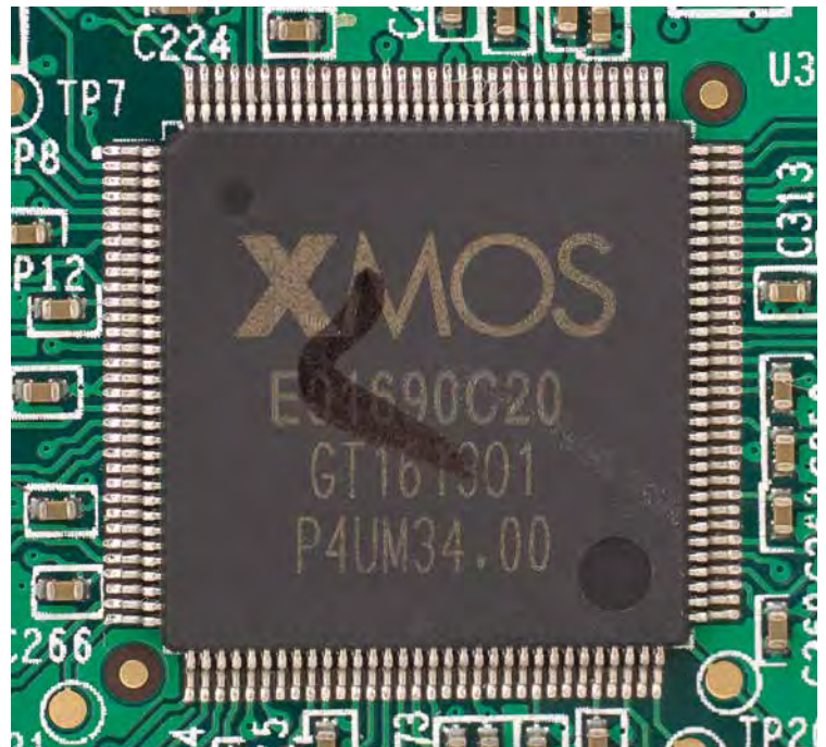
The XMOS DSP is responsible for equalizing the incoming signals, and processes them to ensure optimum sound quality.
