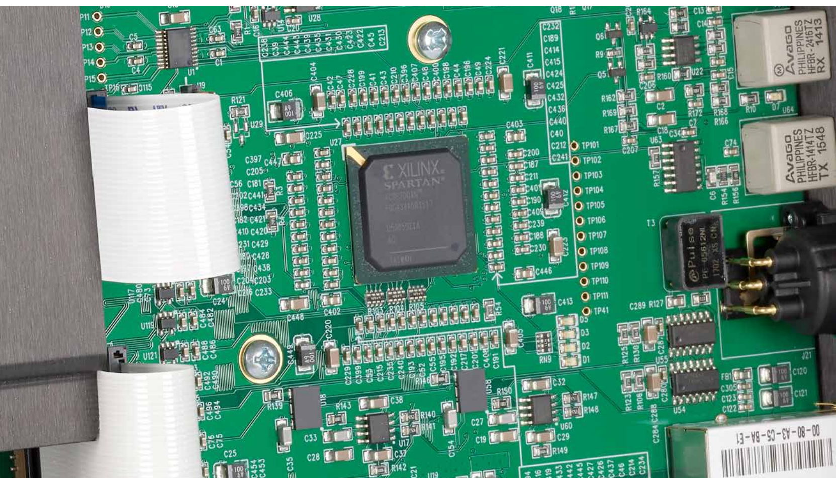
Two FPGAs (field programmable gate arrays) on the digital boards provide upsampling and symmetry; the analog side also has one of the specially programmed ICs.
