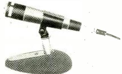
Specifications: dynamic; cardioid dir. pattern; baked enamel finish; output impedance 30/50, 150/250, 20k ohms; freq. resp. 45 to 15,000 cps; length of cable furnished 15 ft.; dimensions—1½" dia., 7¼" long; weight 11 oz. Slip-on adapter mounting. Price, \$72.00. Altec-Lansing.
