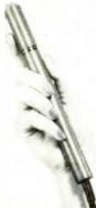
*Specifications:* dynamic; omnidirectional pattern; steel case; non-reflecting gray finish; output impedance 50 or 150 ohms; freq. resp. 40 to 20,000 cps; sensitivity 0.050 (50 ohms), 0.095 (150 ohms) mv/bar; length of cable furnished 25 ft.; dimensions— $\frac{3}{4}$ " dia., 8 $\frac{1}{2}$ " long; weight 7 ozs. Slip-in swivel stand adapter. Price, \$175.00. Shure Bros.
