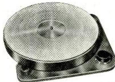
*Specifications:* Speeds—16%, 33 $\frac{1}{3}$ , 45, 78 rpm; rim drive; 4-pole induction motor; turntable diameter, 12" ; turntable weight, 3 lbs; turntable material, aluminum; mat, rubber; wow, 0.2% ; flutter 0.2% ; dimensions of chassis, 12 $\frac{1}{4}$ " x 10 $\frac{1}{2}$ " ; clearance required above mounting board, 1 $\frac{1}{2}$ " ; below, 4" ; controls, speed, power; provision for arm mounting, none; over-all weight, 14 lbs. Price, \$37.50. Lafayette Radio.
