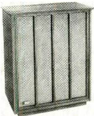
speakers—15" l.f., 8" m.f., 2" h.f.; power handling capacity 65 watts; crossover network L-C air-core coils, continuously variable presence & brilliance controls. Impedance 8 ohms; frequency response ± 2.5 db from 34 to 18k cps; magnet structure weight: l.f., 96 oz.; m.f., 88 oz.; h.f., 88 oz.; voice coil diameters: l.f., 2"; m.f., 1.5"; h.f., 2". Dimensions: 24¾" wide, 30¼" high, 14¾" deep; weight, 80 lbs.; scandinavian walnut \$249.50. Fisher Radio.
