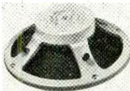
in magnetic design. The use of ceramic magnets in these speakers results in a considerable reduction in weight and depth. Flux density 14,000 lines per square cm, magnet type Ferrobar, total flux 82,000 Maxwells, freq. response 25 to 15,000 cps. Price \$53.99. Richard Allen Sales.
