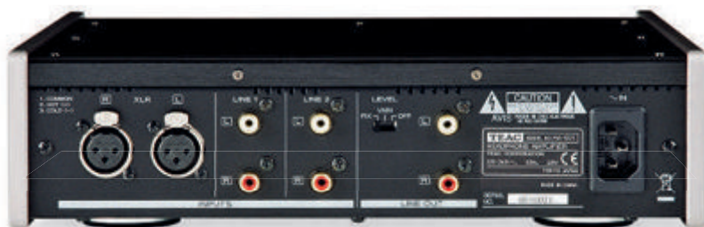
ABOVE: Two unbalanced inputs on phono sockets are complemented by a balanced input on XLRs. Fixed- or variable-level unbalanced output on phonos enables the HA-501 to operate as a simple preamp but for ultimate sound quality is best disabled
