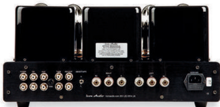
ABOVE: Three line inputs – four with the tape monitor loop – are provided. High/low sensitivity switch at rear allows the integrated to be used as a power amplifier
