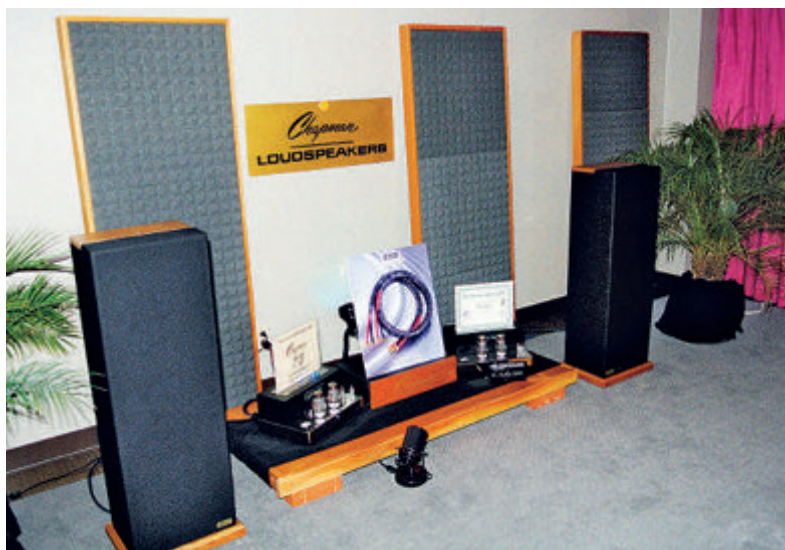
Chapman's T-5 floorstander (US $4995 per pair) contains a 10in woofer with polyamine fibre cone, 5.25in cone midrange and a 1in silk dome tweeter with sealed rear chamber, the mid and tweeter being on a sloped, time-aligned baffle. Enclosure size is 1022x326x254mm (hwd), and the wood finish seen here is solid cherry. www.chapmanaudiosystems.com
