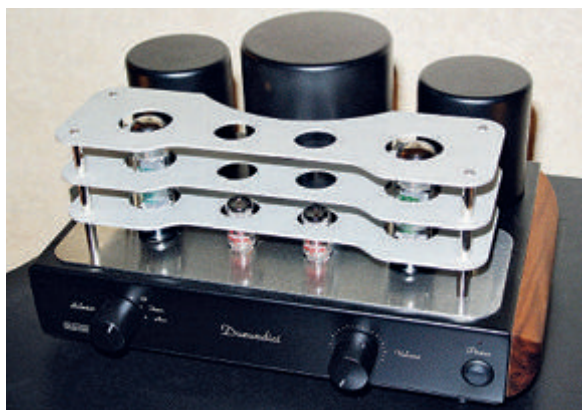
Mastersound of Italy's Dueundici (which is Italian for '211') is a luscious integrated valve amp delivering 2x11W – hence the name – from two EL34s driven by two ECC802s in Class A mode. It provides three line-level inputs, an ALPS Blue potentiometer, autobias, no negative feedback. www.mastersoundas.it
