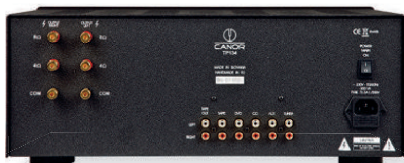
ABOVE: Canor's TP134 has five line inputs and a fixed-level 'Tape' output, all on gold-plated RCA sockets. Speaker binding posts provide 4ohm and 8ohm taps
