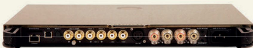
ABOVE: Rear of the Devialet 170 showing USB/Ethernet ins and S/PDIF and AES/EBU outs
