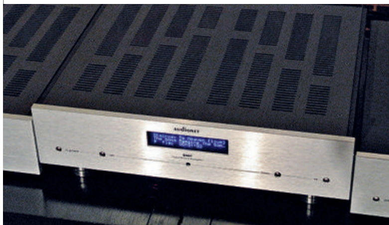
Mastersound of Italy's Dueundici (which is Italian for '211') is a luscious integrated valve amp delivering 2x11W – hence the name – from two EL34s driven by two ECC802s in Class A mode. It provides three line-level inputs, an ALPS Blue potentiometer, autobias, no negative feedback. www.mastersoundas.it
