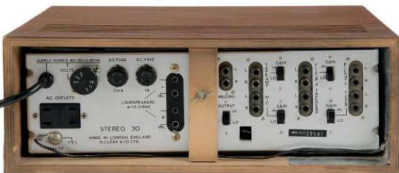
ABOVE: The rear panel is packed with facilities, including a voltage selector for connecting the amp to a range of power supplies; power cable measures 13ft!
