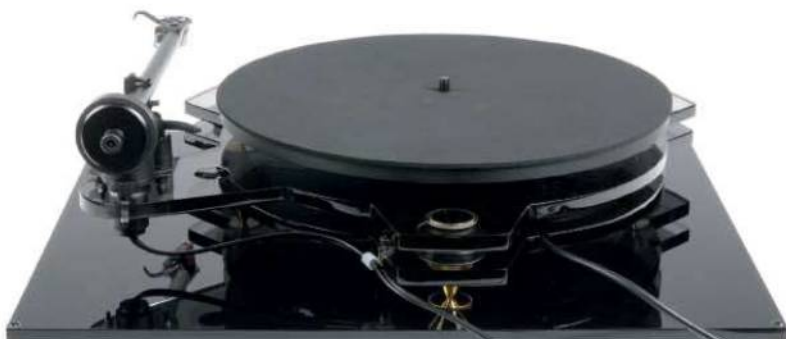
ABOVE: The Rega/Moth tonearm cable is dressed against the subchassis via a P-clip while the power cable for the AC synchronous motor enters from the other side
