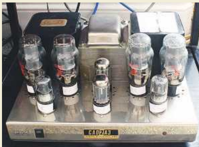
ABOVE: David's Cary Audio Design 2A3 PP power amplifier with its Sovtek 2A3 valves
