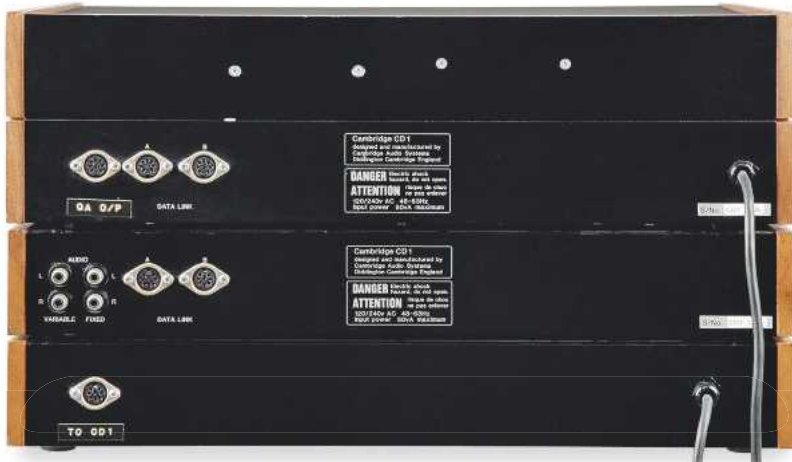
ABOVE: Inter-box connections are made using DIN sockets. The two sets of phono sockets are for analogue outputs, with both fixed and variable options available
