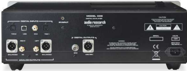
ABOVE: Balanced (XLR) and single-ended (RCA) analogue outputs are joined by USB, optical and coaxial S/PDIF and one AES/EBU digital input. Digital outs are offered too
