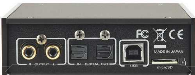
ABOVE: The provision of Toslink digital ins and outs confers real flexibility, while RCA line outs give preamp functionality. USB in is for computer, MicroSD for upgrades
