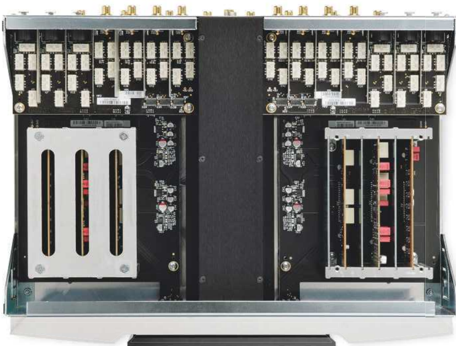
RIGHT: Local relay switching in the preamp proper connects to and from line and MM/MC phono amplifier cards (right channel enclosure opened for clarity in this picture)
