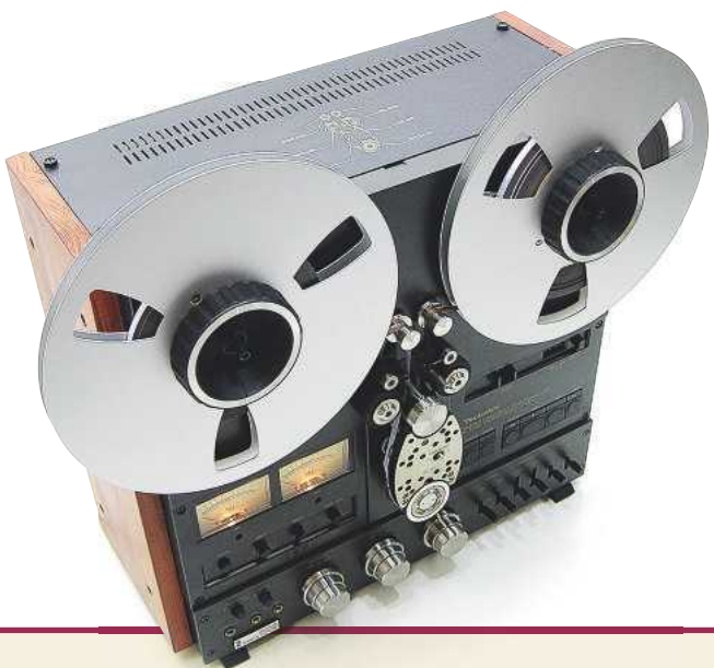
BELOW: Technics' RS1500 literally turned the tape path on its head thanks to the isoloop system
