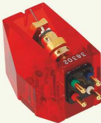
ABOVE: Benz Micro ACE SL with exposed generator set within an acrylic body
