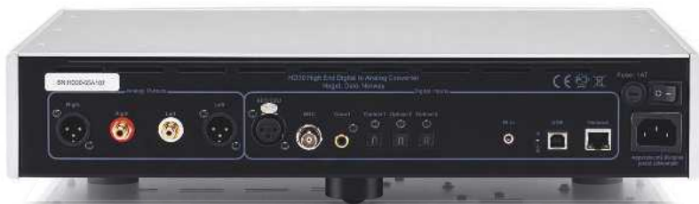
ABOVE: Three optical and two coaxial (BNC and RCA) S/PDIF ins are joined by AES/EBU and USB with an Ethernet port supporting Apple AirPlay and UPnP streaming. Variable (and fixed at volume '101') outputs are available on RCAs and balanced XLRs
