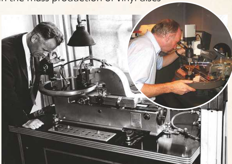
ABOVE: Then and now – a lathe with a diamond stylus cuts a spiral groove into a master disc while (right) cutting a master on a DMM VMS 82 lathe at Abbey Road
