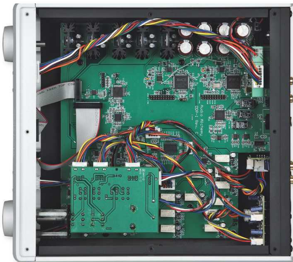
RIGHT: Inside the compact DDP-1 multiple regulated supplies feed the analogue preamp, X MOS-based USB input and a pair of AK's premium, DSD-ready/32-bit AK4399 DACs
