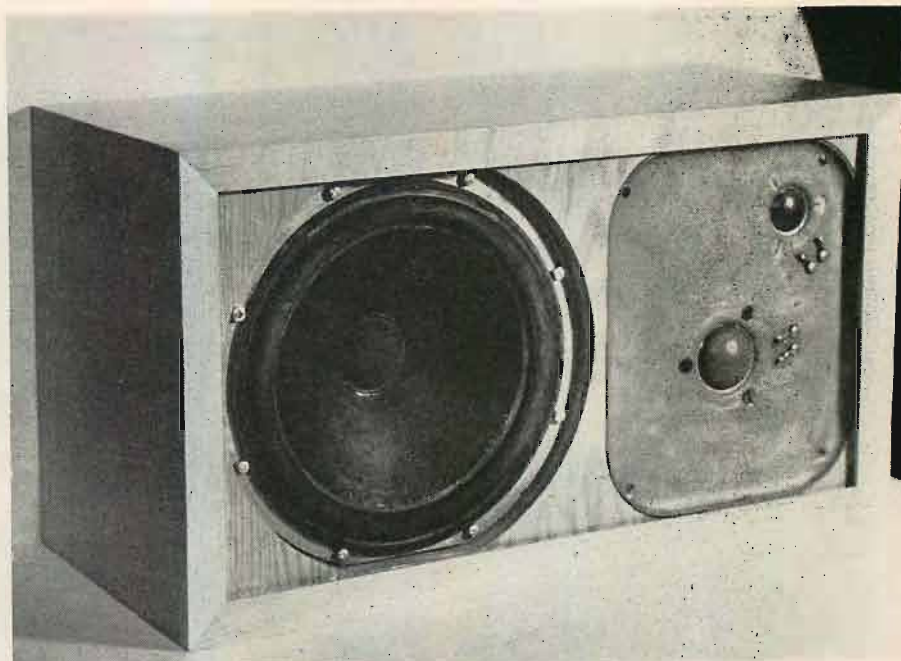
Fig. 9. Prototype of AR-3 speaker system, including AR-1 acoustic suspension woofer and the two tweeters described in this article. (Photo by Bunker.)
