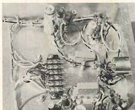
Fig. 7. Arrangement of Vector sockets for amplifier stages.
