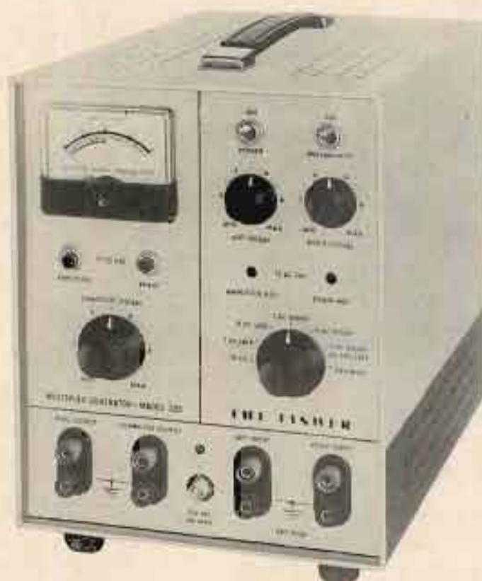
New Fisher Multiplex Generator which provides all the signals required for adapter alignment, both at audio and r.f.
