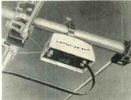
It is recommended by the manufacturer for areas where all signals are less than 20,000 microvolts. The "Red Head" has a bright red amplifier housing for lasting product identification. Winegard Company, Burlington, Iowa. **E-4**
