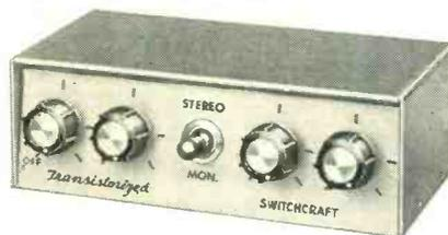
Switchcraft 4-channel high impedance mixers allow you to feed up to 4 signals into a single output to your recorder or amplifier.
