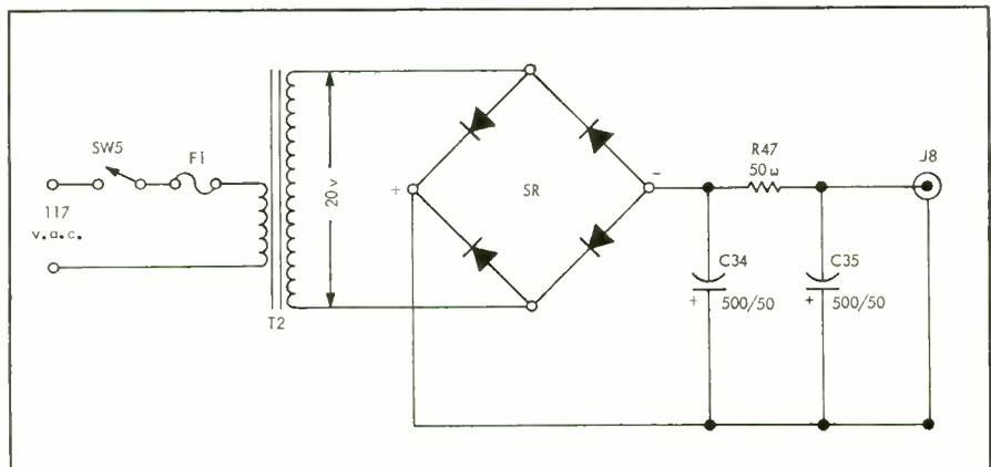
Fig. 5. Schematic of power supply.
