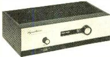
**FM-1**—An outstanding FM tuner with provision for internal insertion of the FMX-3 Stereomatic multiplex integrator. The FM-1 is a super-sensitive (better than 4 μV), drift-free tuner with less than .5% distortion at all usable signal levels. Better than 30 db separation on stereo usage using the FMX-3, and automatic transition to stereo with the visual Stereocator. FM-1 kit \$79.95, wired \$119.95; FMX-3 kit \$29.95; FM-3A (Wired tuner with multiplex), \$169.95.
