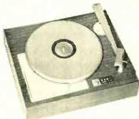
An easy-to-assemble stereo LP turntable kit of professional quality and performance. Rumble better than 50 DB down . . . flutter 0.08% . . . wow 0.2%. Polyurethane drive belt; hysteresis-synchronous drive motor.
