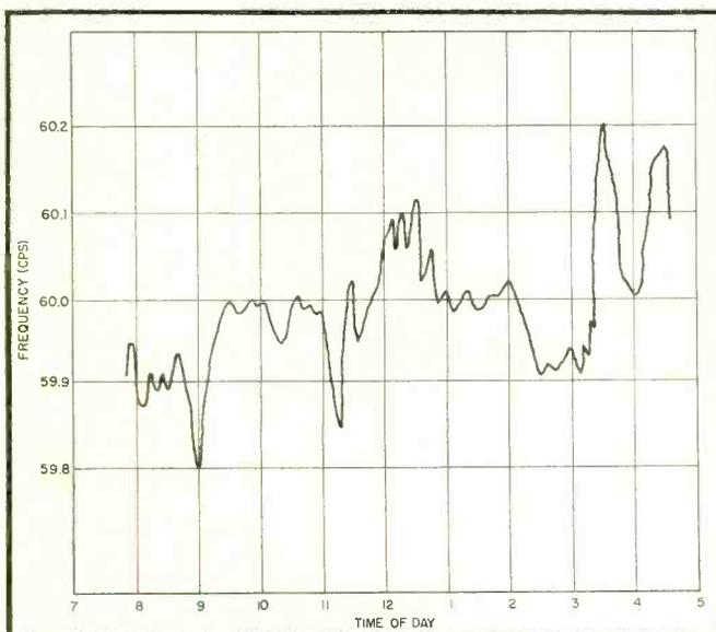
Fig. 5 (left). Measured frequency variation of a 60-cps line; points on the curve represent average values for one-minute intervals. Frequency variation was less than 0.1 cps for 75 per cent of the time, and less than 0.05 cps for 50 per cent of the time.
