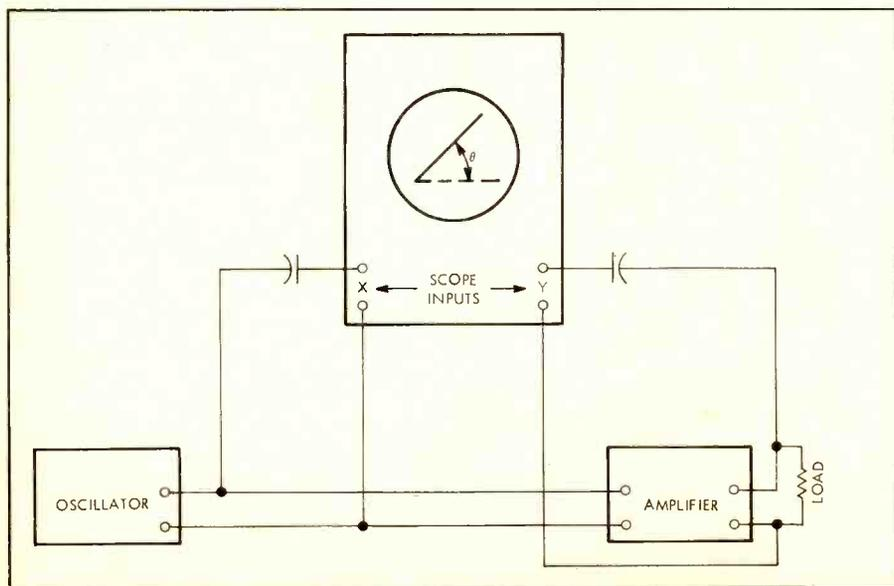
Fig. 1. Typical connections to 'scope from output and input of amplifier to make the observations described in this article.
