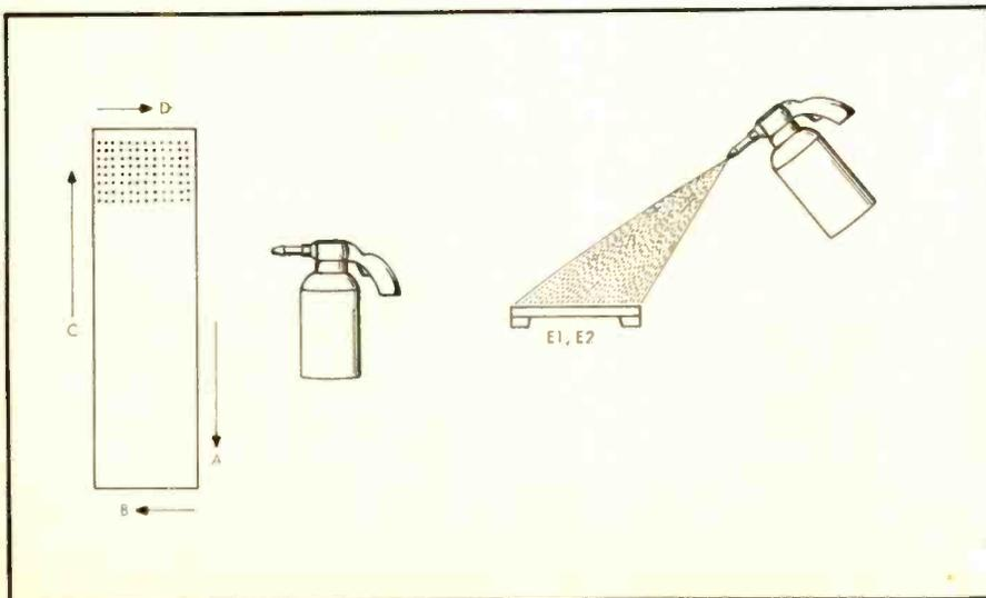
Fig. 8. Method of spraying varnish.
