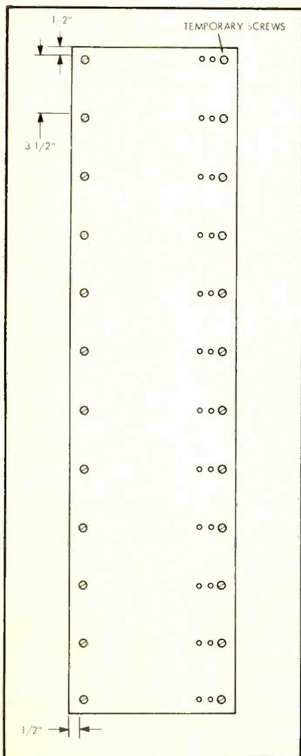
Fig. 3. Layout of mounting holes. Drill holes through electrodes two rows at a time and then use temporary screws to hold new row down.
