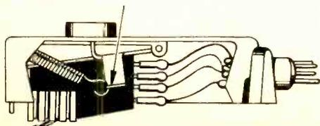
Fig. 5. Cutaway view of the Shure Gard-A-Matic series of cartridges.
