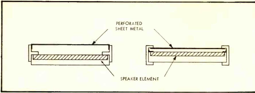
Fig. 11. Completed speaker element must be mounted in a protective enclosure.
