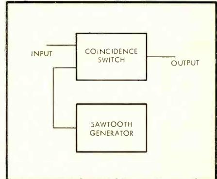
Fig. 6. Oscillator-modulator.
