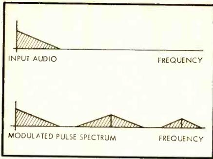
Fig. 3. Modulated pulse spectrum.
