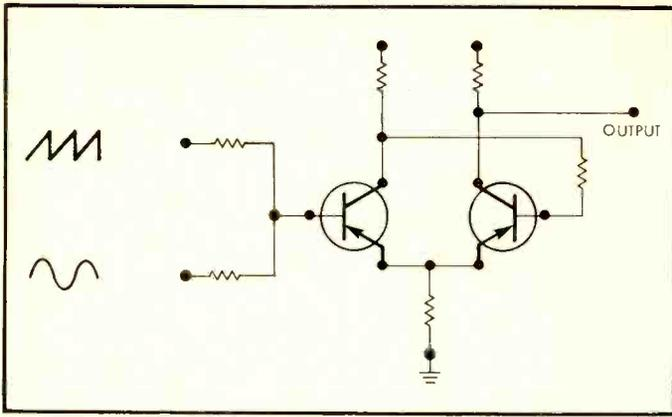
Fig. 10. Schmitt trigger circuit.
