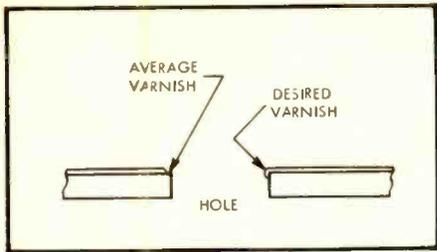
Fig. 7. Varnish should cover edge of hole as shown at right.
