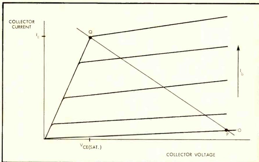
Fig. 2. Transistor characteristics and load line.
