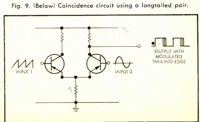
Fig. 9. (Below) Coincidence circuit using a longtailed pair.
