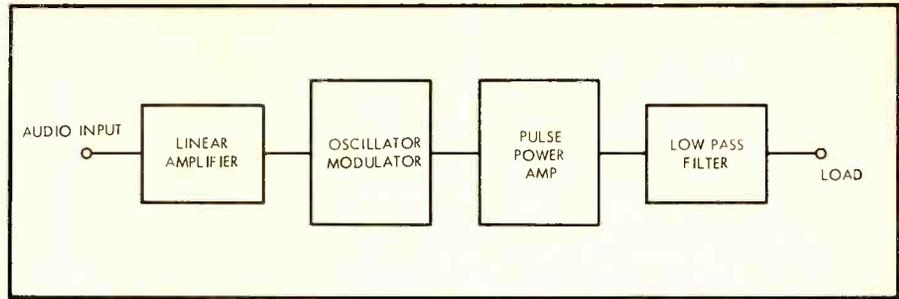
Fig. 5. Block diagram of modulated-pulse audio amplifier.
