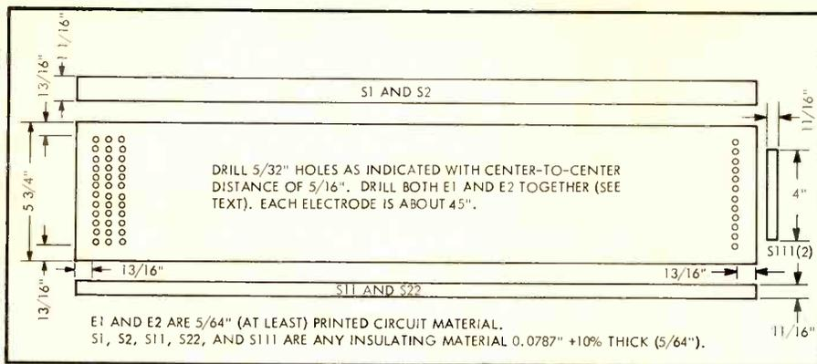
Fig. 2. Dimensions and hole pattern of both electrodes and dimensions of the spacers. Only one each of the electrodes and spacers are shown; two are required.
