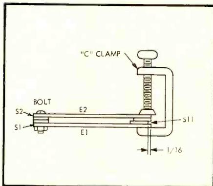
Fig. 5. Bolt  $E_1$  to  $E_2$  with  $S_1$  facing  $S_2$  and clamp  $S_{11}$  in position indented  $1/16$  in. as shown.
