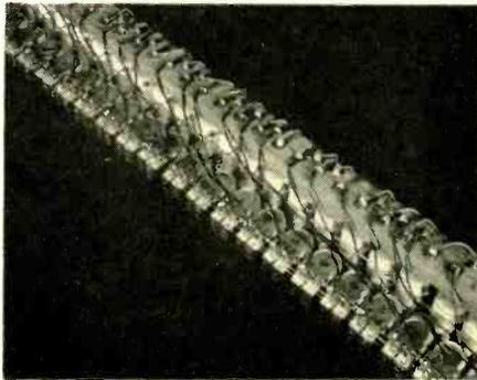
Fig. 2. Part of a bank of relays used to produce the time-sequenced key closures. Adjustment of the contacts can produce any desired timing in the sounding order of the mixture.
