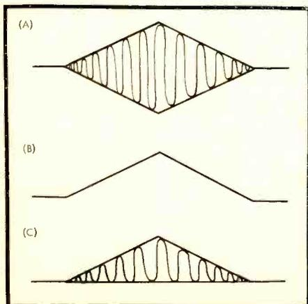
Fig. 1. Combining signal and envelope to produce a composite signal.
