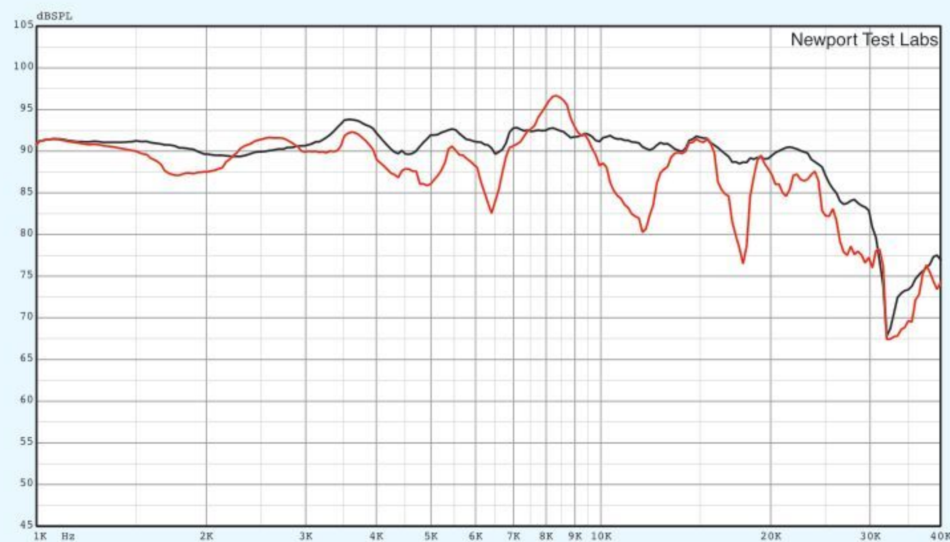
Graph 2: Anechoic high-frequency response, on axis, with grille off (black trace) and with grille on (red trace).
