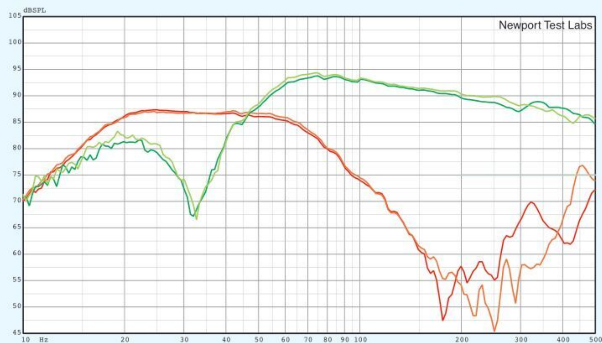
Graph 3: Low frequency response of bass reflex ports (red/orange traces) and bass drivers (dark/light green). Nearfield acquisition. Port/woofer levels not compensated for differences in radiating areas.
