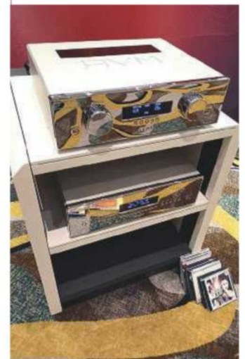
Here's AVM's Ovation 8.3 integrated amplifier above its 8.2 CD player. The amp is a Class A/AB design rated at 200W per channel into 8ohm and offers Bluetooth 4.2 connectivity. The slot-loading disc player, meanwhile, offers six digital inputs and employs tubes in its analogue output stage filter. www.avm.audio
