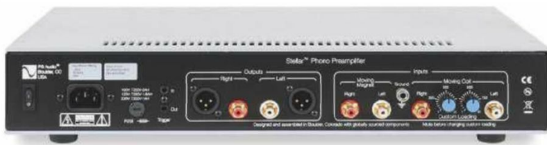
ABOVE: Separate MM and MC inputs will support two tonearms simultaneously while the MC input also includes continuously variable loading (10ohm-1kohm). RIAA eq'd outputs are offered on RCAs and balanced XLRs
