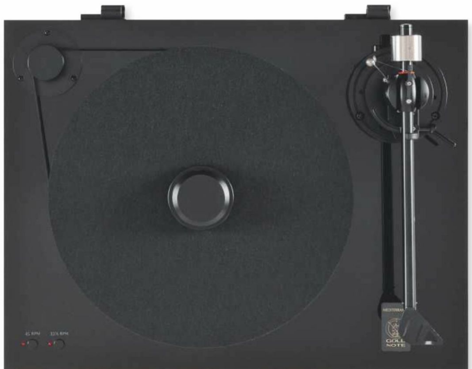
RIGHT: Top-down view highlights the 9in B-5.1 tonearm which uses four micro ball-bearings by GRW (Germany). The AC motor is Swiss and drives the 45mm-thick POM platter via a round-section belt. Felt mat is supplied but optional
