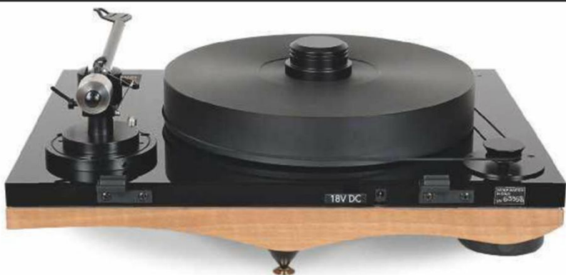
ABOVE: Supported on three inverted cone feet, the Mediterraneo accepts an 18V feed from a supplied AC/DC unit or from the optional (£864) PST-10 outboard PSU [see below]. Phono leads use a standard DIN connection into the base of the arm
