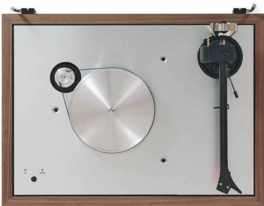
RIGHT: The Evo version of the Classic features a heavier sub-platter, machined from the same grade of aluminium alloy as the main platter. Speed control – 33.33/45/78rpm – is electronic
