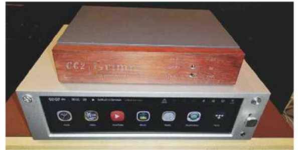
The RS201 is made in Korea by Seoul-based company Rose and it seems there's little this all-in-one network player can't do thanks to its built-in amp, ES9018K2M 32-bit DAC from Sabre and 4K video processor that outputs content via HDMI. www.hifirose.com
