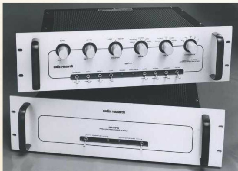
LEFT: A hybrid tube/FET stereo preamplifier, the SP-11's control unit (top) housed six 6DJ8/ECC88 valves while the separate SP-11PS power supply was a purely solid-state design. The two chassis were connected via a supplied 4ft-long interconnect cable
