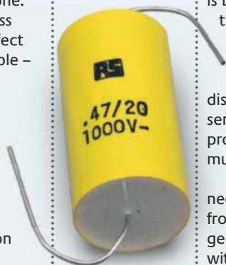
BELOW: Fig 8 – a high-voltage polypropylene film capacitor. In the 1980s it became common to see these used in parallel with reservoir capacitors
