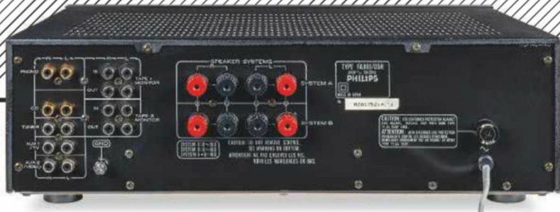
ABOVE: Gold-plated RCAs serve MM/MC phono and CD inputs with nickel-plated RCAs for three line and two tape inputs. Two sets of speaker cable binding posts (not 4mm) are switched via relays controlled by buttons on the fascia [see p123]
