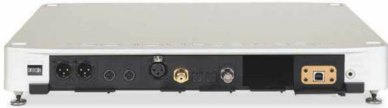
ABOVE: Our Discrete DAC was supplied with two PSUs, the 2x2 DC supplies carried via two umbilicals. Input modules included USB-B (768kHz/32-bit; DSD512), coaxial/optical (S/PDIF) and wired Ethernet (768kHz/32-bit; DSD256 – removed in this picture). Balanced preamp outs may be configured for fixed or variable output
