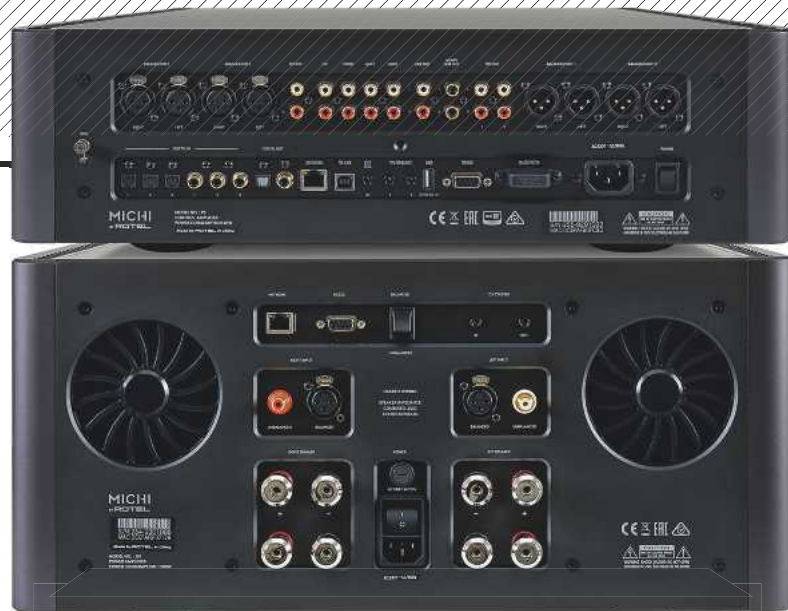
ABOVE: The P5 preamp [top] offers MM/MC phono and six line ins (two balanced on XLR), a fixed line out, two sub outs, four preamp outs (two on XLR). Digital ins include six S/PDIF (three coax/three optical), USB-B and wireless BT. Network port is for control only and USB-A for charging. The S5 power amp has balanced (XLR) and RCA ins, trigger connections and two sets of substantial 4mm speaker cable binding posts
