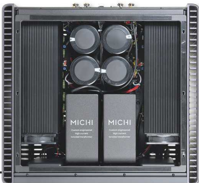
LEFT: The S5 is dual-mono right from the 2.2kVA epoxy resin-filled transformers and two UK-sourced PSU reservoir caps (47,000µF each) per channel. Each Class A/B output stage has eight pairs of high-current power transistors on a fan-assisted heat pipe
