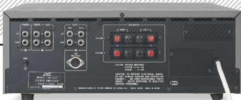
ABOVE: Nickel-plated RCAs serve MM phono, tuner and aux inputs, with another set of RCAs, duplicated by a 5-pin DIN, to service a tape loop. Two sets of speaker cable screw terminals are switched, individually or together, via a lever on the fascia [p114]
