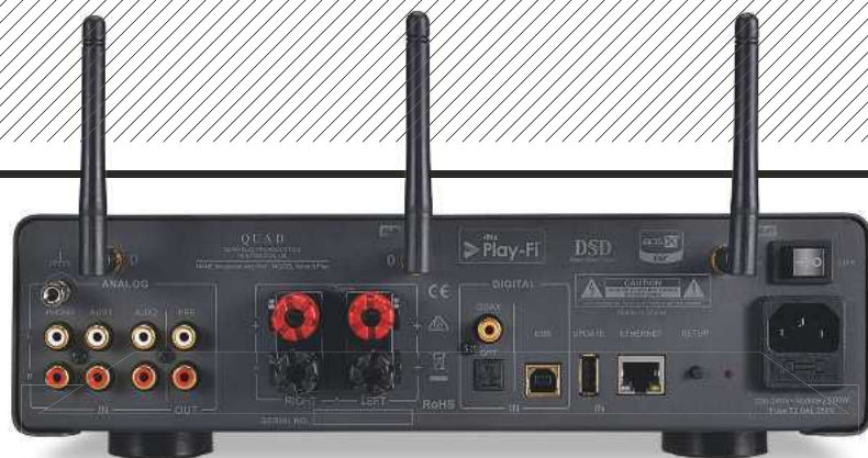
ABOVE: With Ethernet and Wi-Fi added to the BT 'inputs', there are just two S/PDIF inputs here (one coax, one optical), plus asynchronous USB-B and two RCA line ins, one MM phono, one preamp out and 4mm speaker terminals
