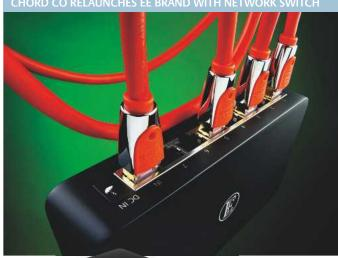
Cable specialist The Chord Company has launched its first ever electronics component, and in doing so has revitalised the brand name English Electric (to avoid confusion with the entirely separate Chord Electronics Ltd). The 8Switch is an eight-port Gigabit Ethernet hub designed for network audio streaming, and boasts a machined aluminium chassis and resonance-damping feet
