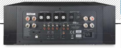
ABOVE: Five line ins (three on RCAs, two balanced on XLRs), USB-B and pairs of coax/ optical digital ins are joined by balanced and single-ended pre outs (XLR/RCA), one fixed line out (RCA) and coax/optical digital outs. There are two sets of floating (live negative and positive) 4mm speaker outlets per channel for easy bi-wiring
