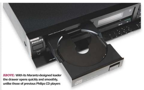
were built on a sturdy die-cast alloy chassis, but this had now been replaced with lightweight plastic mouldings as part of the CD/CD (Compact Disc/Cost Down) project.
