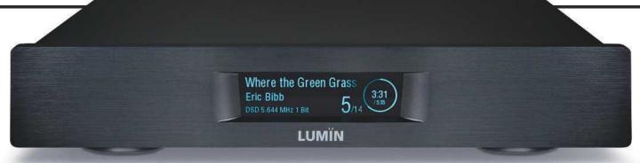
the former being preferable given the all-balanced internal layout, offering a choice of 'Normal' or 'Low' level, and a volume control governed via the app. In addition there's a single BNC digital output, limited to 192kHz/24-bit and DSD64 via DoP – and that's just about all you get.
