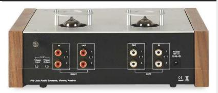
ABOVE: The Tube Box DS2 will accommodate two turntables/cartridges with separate, but switched, RCA inputs and outputs. 12V triggering facilitates a degree of system automation while the 18V wall-wart PSU invites user-driven upgrades
