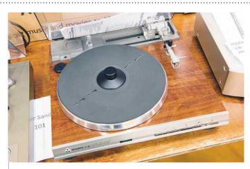
This one drew the crowds, being a super-rare, linear-tracking, direct-drive, quartz-controlled Mitsubishi LT-20 turntable, fitted with an Audio-Technica cartridge and supplied with record puck. Fully overhauled, with instruction booklet and service manual, this utterly clean example was being offered for £350, or around £100 below a lesser LT-20 seen online.
