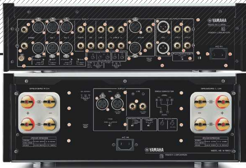
ABOVE: The preamp [top] offers an MM/MC phono input, six line ins (four on RCAs and two on XLRs), two direct inputs (XLR and RCA) and three sets of main outputs (on RCAs and XLRs). The (bridgeable) power amp [below] has inputs on RCAs and XLRs, and two pairs of loudspeaker outputs on gold-plated 4mm cable binding posts
