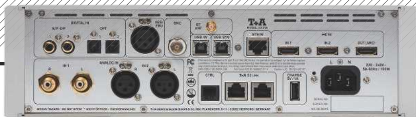
ABOVE: Digital inputs span S/PDIF (two coaxial, one BNC, two optical), AES/EBU (on XLR), USB-B for computer connection, optional £480 HDMI module for BD players, and wireless Bluetooth. Analogue inputs are on RCAs and balanced XLRs
