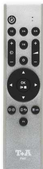
LEFT: The legends on T+A's rechargeable FM8 remote are not entirely intuitive but include input selection, volume and menu navigation
