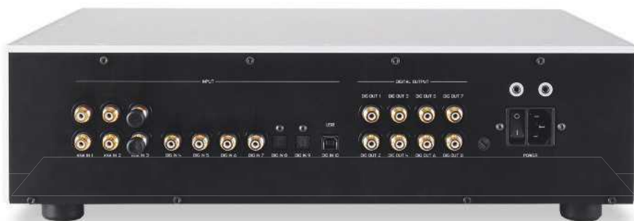
ABOVE: Three stereo analogue line ins are joined by six S/PDIF digital ins (four coaxial/two optical that accept 96kHz LPCM) and one USB-B (rated at 48kHz). Four sets of configurable (stereo or mono) S/PDIF digital outputs feed the left and right Prana speakers, respectively, at 96kHz/24-bit
