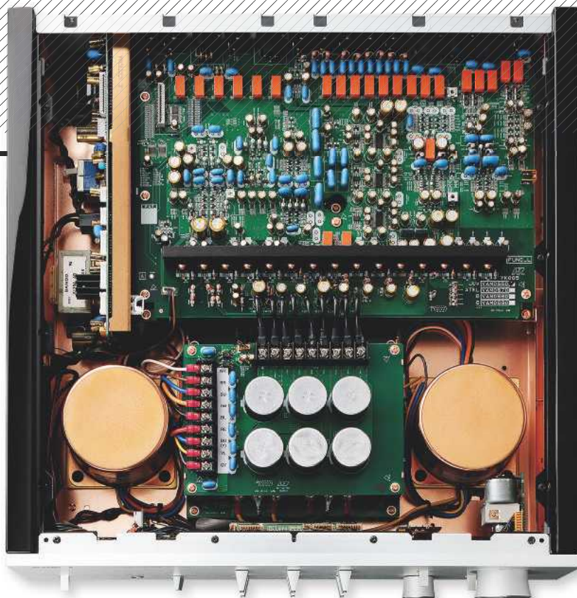
ABOVE: The fully balanced, dual-mono preamp features mirror-imaged L/R circuit boards, one atop the other [top]. Separate L/R PSUs are fed from two screened toroidal transformers [lower left/right]
