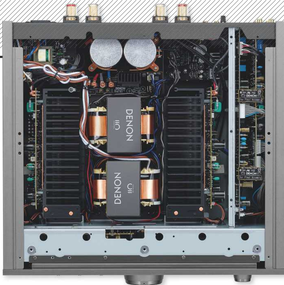
ABOVE: Transformers [centre] and 71V/ 12,000µF reservoir caps [top] form the core of the PSU that feeds a very low-noise preamp [far right] and dual-mono FET power amps [on heatsinks]. The innards look like those of the PMA-2500NE, but the two-stage single-ended amp is inspired by the PMA-SX11
