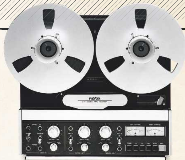
ABOVE: The Revox B77 introduced a number of improvements over its A77 predecessor, most notably to the head block, motor and electronics. It would go on to be produced in over 50 variants
