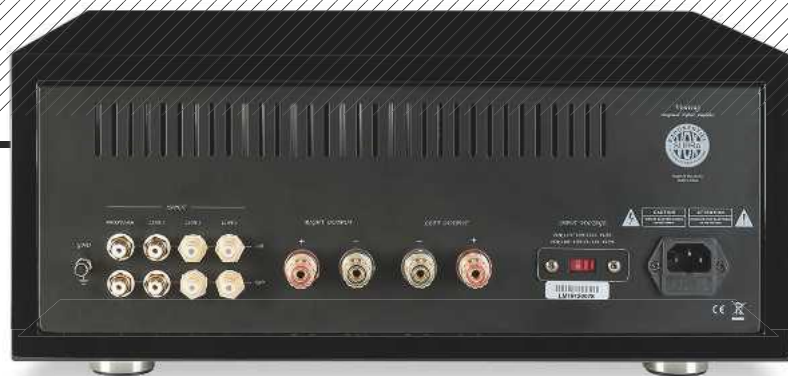
ABOVE: No 'digital' here – just one MM phono and three line inputs on RCAs with single sets of switched speaker outputs on 4mm sockets/binding posts
