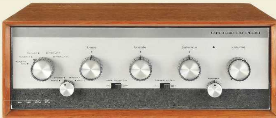
ABOVE: Leak's 'Plus' version of its Stereo 30 amp used silicon rather than germanium transistors
