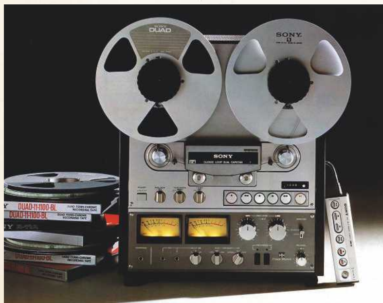
LEFT: The Sony TC766-2 boasted the company's tried-and-tested dual-capstan tape transport along with its own ferrite magnetic heads. The tape path was complex, with damped tension arms and rollers guiding the tape along its way
