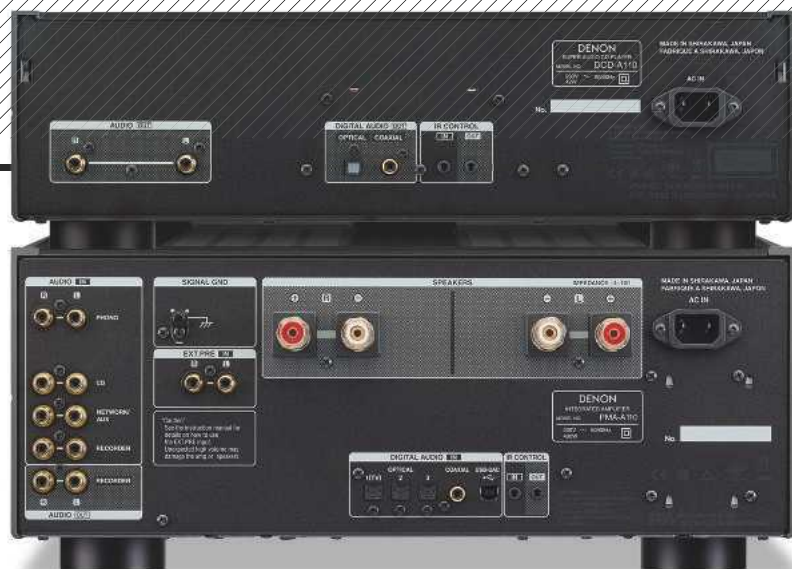
ABOVE: CD/SACD player [top] has optical/coaxial digital outs and analogue outs on RCAs. Amp [below] has MM/MC, a processor and three line ins, a power amp input, three optical, coax and USB digital inputs plus one set of 4mm speaker binding posts
