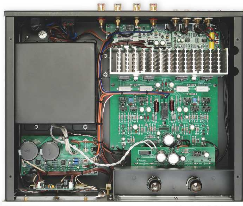
RIGHT: Shielded transformer and PSU [left] occupy a large portion of the enclosure. Triode line stage [lower right] feeds power amp with pairs of devices on heatsink [top]. MM phono stage sits right behind the RCAs [top right]
