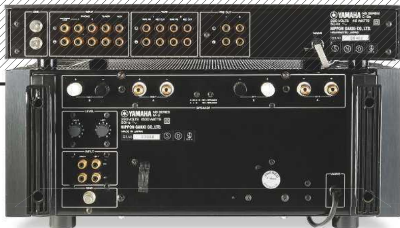
ABOVE: There's no shortage of inputs on the C-2a while the M-2 [below] has two sets of speaker outputs. The C-2a's leftmost RCAs are for Phono 1 capacitance loading plugs, and the M-2 offers variable input sensitivity plus AC and DC coupled inputs
