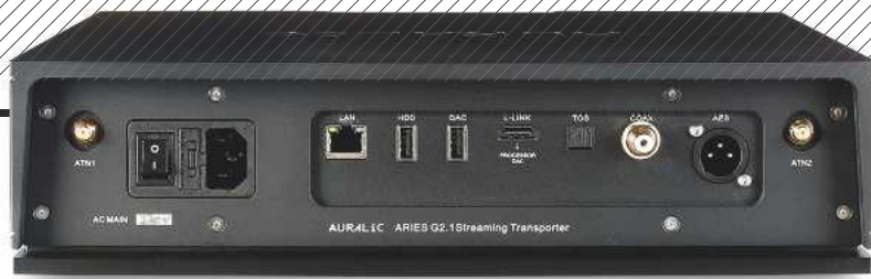
ABOVE: Digital only – the Aries G2.1 offers wired/wireless network control/streaming ins plus access to more music via internal and an external (HDD) USB drives. DSD512/384kHz outs are on USB-A, I 2 S (via HDMI) and DSD64/192kHz on Toslink, coax and AES
