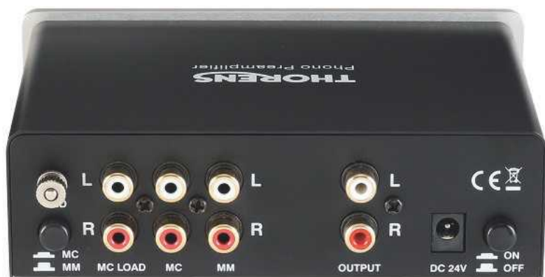
ABOVE: The MM-008 will accommodate separate MM and MC pick-ups via switched, RCA inputs. MC loading is achieved via supplied phono plugs containing 10, 100ohm and 1kohm resistors while the 24V wall-wart PSU invites user-driven upgrades
