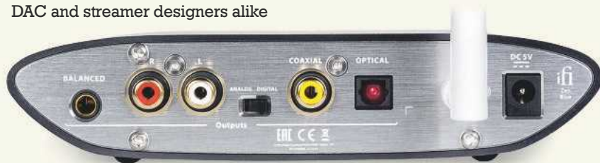
ABOVE: Rear of iFi Audio's ZEN Blue DAC with its Toslink optical output glowing red
