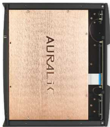
ABOVE: Hidden under the top-plate and screening the digital electronics within is a luxurious, branded copper enclosure
