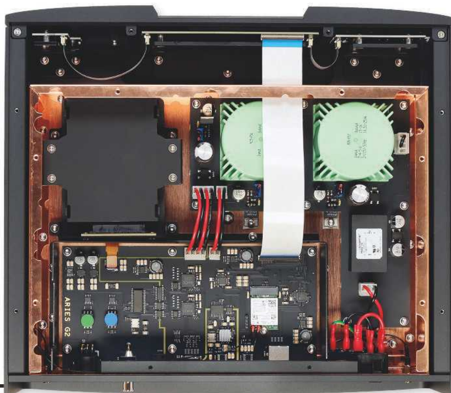
RIGHT: One linear PSU [top right] feeds an Intel Tri-Band Wi-Fi/BT module [lower right], XMOS USB solution [lower middle], Cirrus CS8406 digital transmitter and clocks on the 'Tesla' PCB. Second PSU feeds display and storage [top centre]
