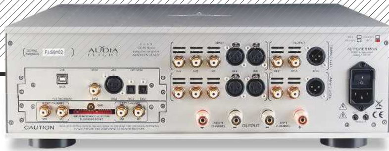
ABOVE: Our sample was equipped with the new MM/MC phono [lower left] and digital modules, the latter with USB-B, AES, two optical and one coax input [upper left]. Default line ins include three on RCAs, two balanced on XLRs with a tape out and pre outs on XLR/RCAs. Single, switched 4mm speaker outlets are fitted
