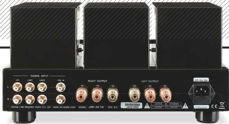
ABOVE: Very straightforward – just three line and a direct (power amp) input on RCAs with 4mm speaker cable outlets wired via 8ohm and 4ohm transformer taps
