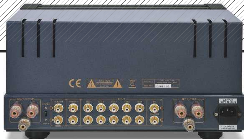
ABOVE: The EVO 300 offers five line inputs, an HT bypass, tape out and sub/mono line outs with a trio of 4mm speaker outputs per channel fed from 8ohm and 4ohm transformer taps, respectively. Optional MM phono module is not shown here
