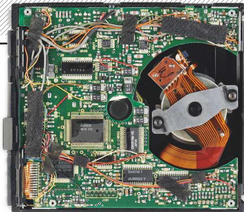
ABOVE: Internal view shows the densely-packed PCB. Note that the word 'Sony' has been blacked out on the major ICs – including the CX23035 decoder [large central IC], the CXK5816 static RAM [centre, right] and CX20133 DAC [top left]
