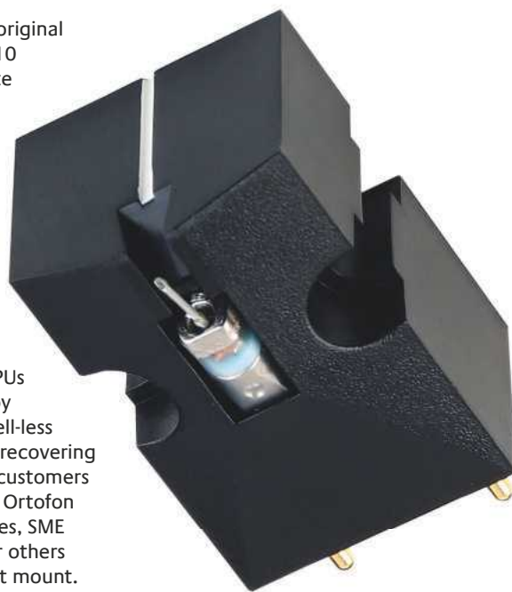
ABOVE: No fancy materials here as a tried-and-tested double-walled aluminium cantilever is fitted with a solid diamond stylus featuring a 0.5mm spherical tip
