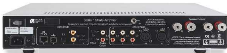
ABOVE: Three line ins (two on RCAs, one balanced on XLR) are joined by an HT bypass, preamp output and speaker outputs on 4mm terminals. Digital ins include wired/wireless Ethernet, USB-B, optical, two coaxial and PS on an HDMI socket
