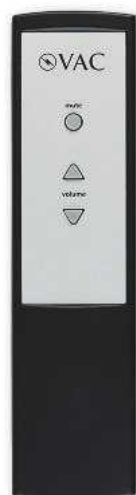
LEFT: VAC's heavyweight alloy remote offers control over the motorised (belt-driven) volume control and mute, but not input selection
