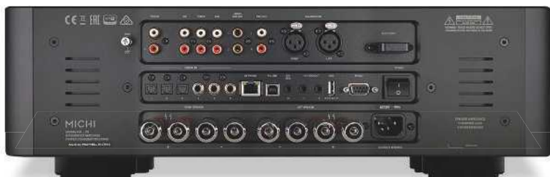
ABOVE: The X3 offers MM phono, one balanced (XLR) and three RCA line ins; sub and preamp outs; three optical, three coaxial and one USB-B digital ins; trigger, RS232 and network control ports plus two sets of substantial 4mm speaker cable binding posts
