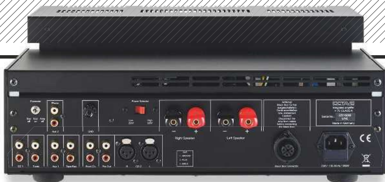
ABOVE: The V70 offers optional MM or MC phono, four line inputs (one balanced on XLRs), a tape input, fixed and preamp line outs plus speaker outputs rated for 4-16ohm loads. Lockable socket is for Octave's optional 'Black Box' capacitor bank
