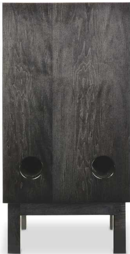
LEFT: Two 75mm reflex ports extend bass below 40Hz. The speaker locates into its matching stand via two wooden struts fitted to the underside of the cabinet [see below]
