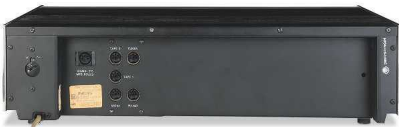
ABOVE: DIN connectors and outputs for use with MFB speakers are on the left while the sunshine logo on the far right indicates the design is suitable for use in all climates
