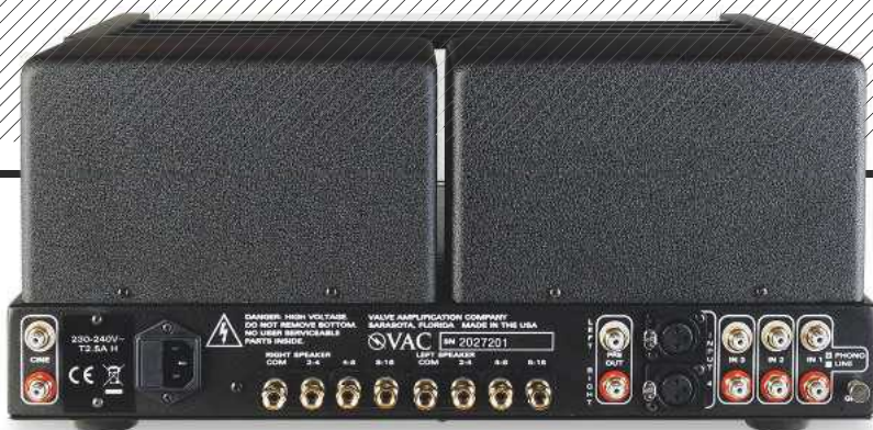
ABOVE: Balanced (XLR), three single-ended (RCA) inputs (one used for MM/MC here) and a direct (HT) input are joined by a preamp output (RCA) and choice of 2-4ohm, 4-8ohm and 8-16ohm speaker outputs on 4mm Cardas cable terminals
