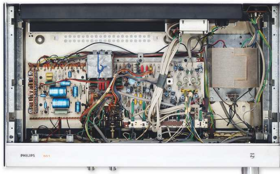
LEFT: Mostly Philips-made components are used in the RH 551. The space [top left] would have accommodated the power amplifier section of the related RH 521 integrated model
