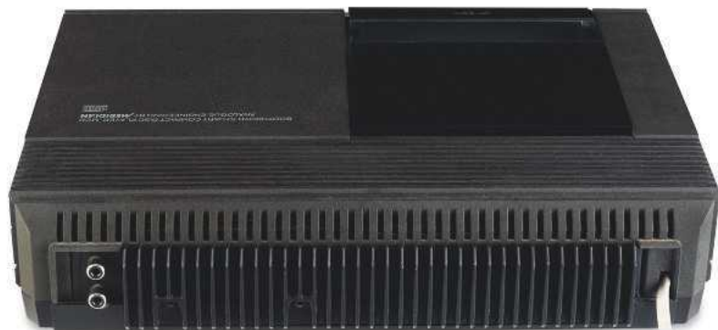
ABOVE: Rear of MCD shows heatsink that forms part of the die-cast Philips chassis. RCA output sockets are not colour-coded, and (black) L/R labels are barely visible
