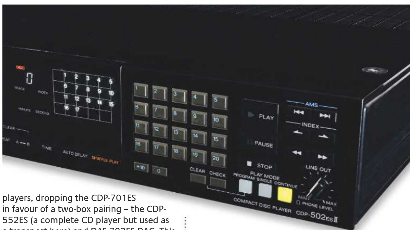
ABOVE: Buttons galore, but it all makes logical sense. The three illuminated 'Play Mode' keys are particularly well thought out and useful
