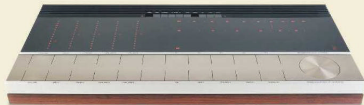
ABOVE: B&O's Beomaster 6000 4Channel receiver packed an SQ decoder for quadraphonic sound while its cosmetics would later see it displayed in the New York Museum of Modern Art
