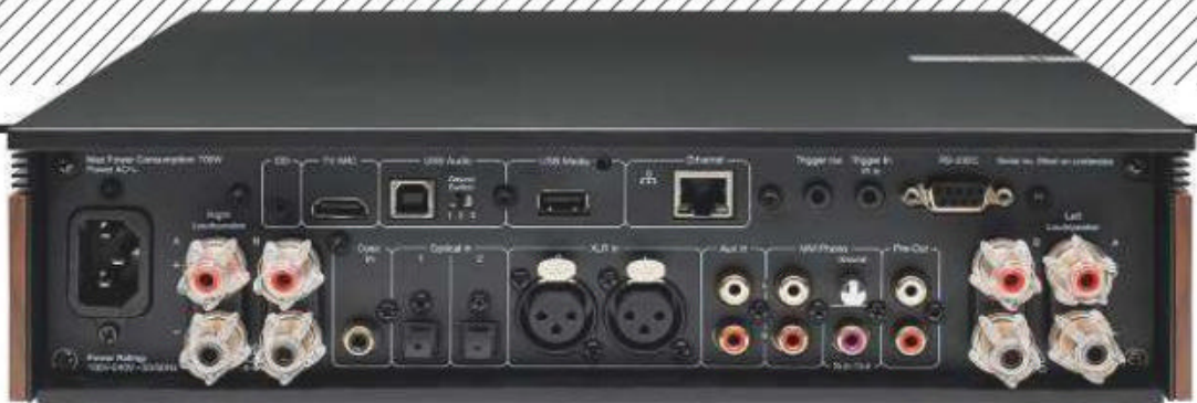
ABOVE: Analogue line ins on RCAs and XLRs are joined by MM phono, two Toslink optical, coaxial, USB-A (for HDD connection), USB-B and wired Ethernet (both 384kHz/32-bit and DSD256) and, inside, Wi-Fi/Bluetooth (aptX HD – 48kHz/24-bit). Pre outs (RCAs) sit alongside two sets of 4mm speaker cable binding posts and 12V triggers
