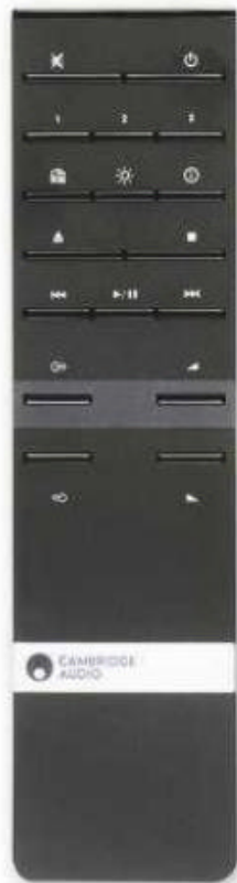
LEFT: Cambridge Audio's latest remote offers access to input, presets, display info, volume, A+B speaker and headphone switching
