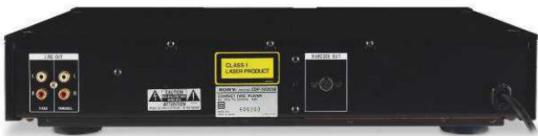
ABOVE: Two sets of single-ended outs were provided on RCAs – one fixed level, the other variable. Subcode out was a forerunner of the industry-standard digital output
