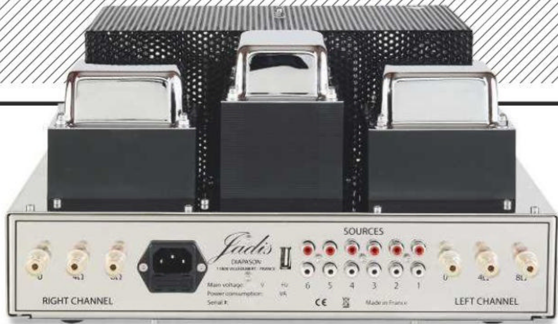
ABOVE: Six single-ended line ins on RCAs are joined by an optional 48kHz/16-bit USB-A (smartphone, etc) connection. Speaker taps for 8ohm and 4ohm nominal loads are offered on 4mm cable binding posts [boxout, p49]. Note cage in place over tubes
